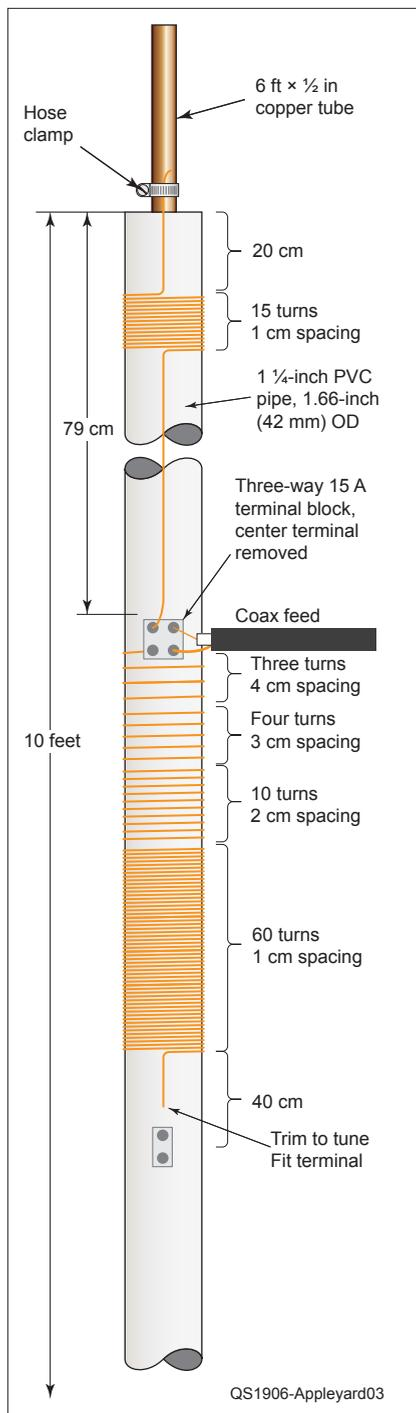
Figure 2 — Details of the dual coil assembly.
