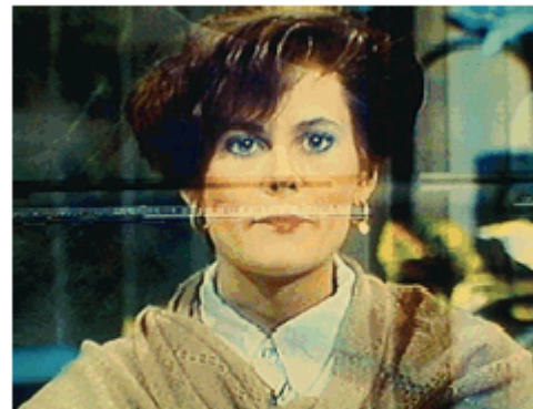
Picture 4: Co-channel Interference
