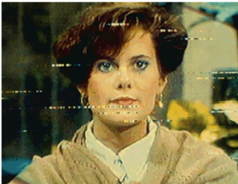
Picture 7: Electrical Interference -- low noise
