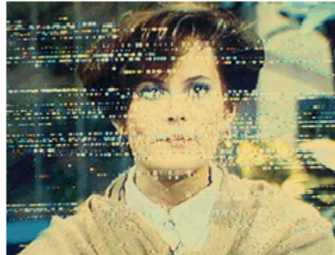
Picture 6: Electrical Interference -- very noisy (hair dryer)
