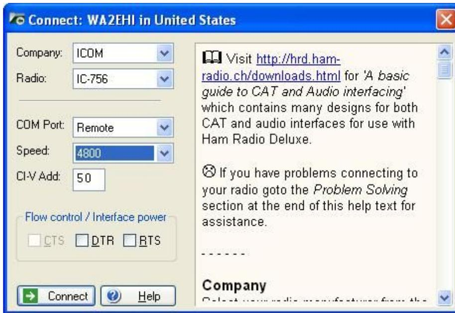
**Figure 6 – Setting Up a Radio for Remote Access**
