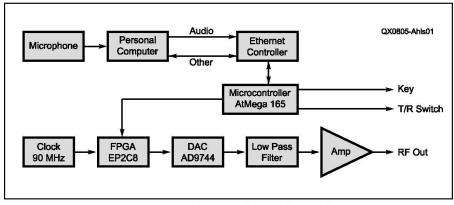
Figure 1 — This is a block diagram of the exciter.
