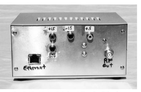
Figure 4 — This photo shows the back panel of the exciter, with the various input/output connectors.
