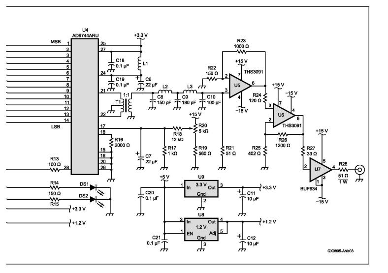
will appear at the output, and any clock jitter will appear as phase noise. You could build your own crystal clock, and if you do I suggest using the differential clock inputs on the FPGA. If you use a CMOS clock oscillator, as I do, avoid those meant for general use, and find one specifically designed for communications use — one with a specified jitter. For DAC use, the clock is a big deal.
