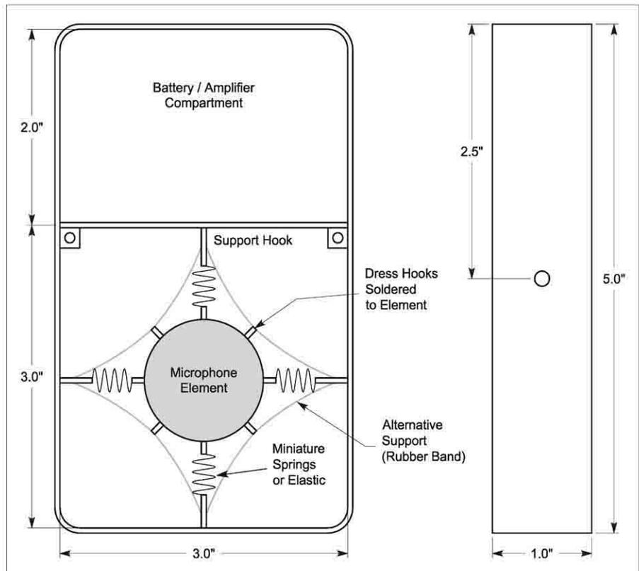
**Figure 9—The dimensions of the microphone housing example. Note that the element is suspended by hooks and elastic. An alternative element support can be a rubber band, also shown. Use either method for support.**
