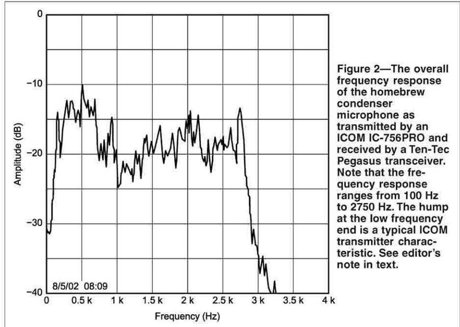
Figure 2—The overall frequency response of the homebrew condenser microphone as transmitted by an ICOM IC-756PRO and received by a Ten-Tec Pegasus transceiver. Note that the frequency response ranges from 100 Hz to 2750 Hz. The hump at the low frequency end is a typical ICOM transmitter characteristic. See editor's note in text.
