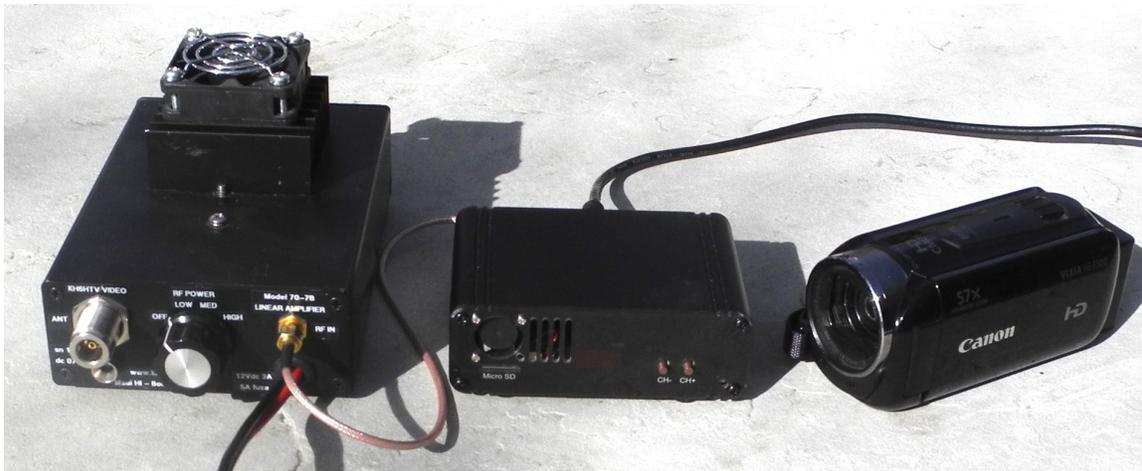
Fig. 22 A complete 70 cm, 3 Watt, DVB-T Transmitter. It consists of a KH6HTV Video, model 70-7B linear rf power amplifier, a Hi-Des model HV-320E modulator, and a Canon camcorder,
