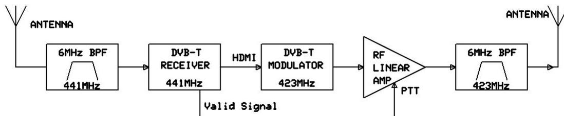
Fig. 28 A 70cm, Digital TV Repeater, Block Diagram
