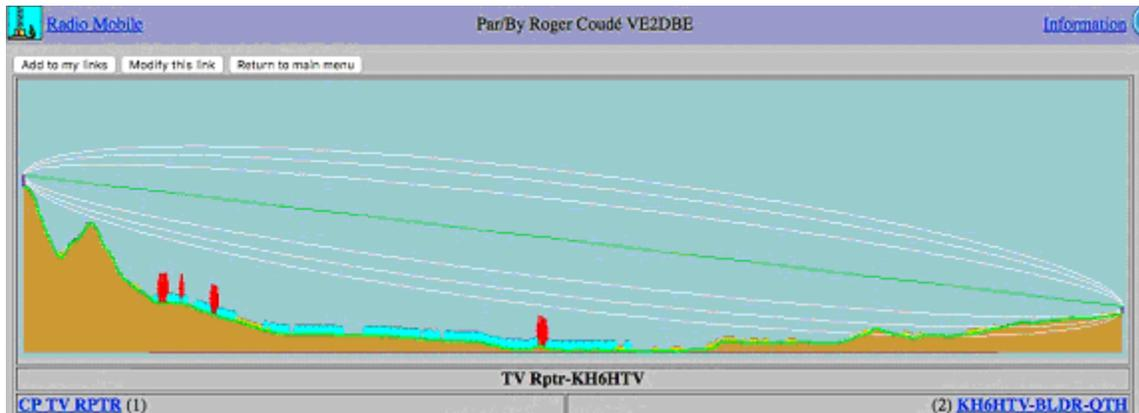
Fig. 25 Typical RF path profile generated by *Radio Mobile*. ATV repeater to KH6HTV QTH, 5.3 mile path shown.
