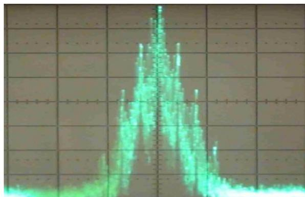
Fig. 12 Typical amateur FM-TV spectrum 10dB/div &amp; 10MHz/div
