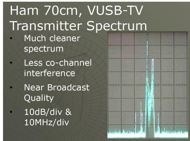
Fig. 11 Spectrum from an amateur VUSB-TV transmitter using a CATV modulator
