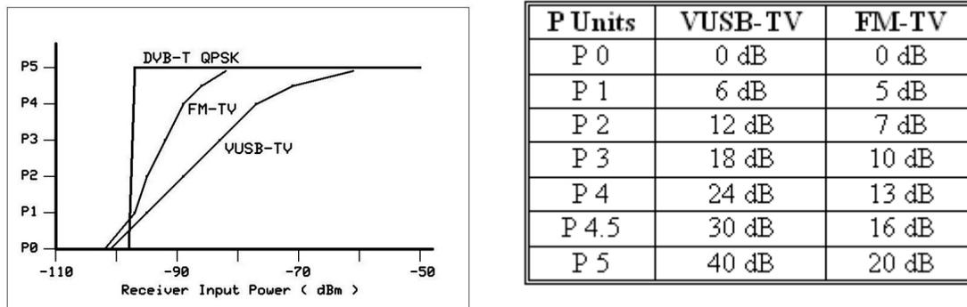
Fig. 8 P Units vs. RF S/N for VUSB, FM TV & DTV Signals
