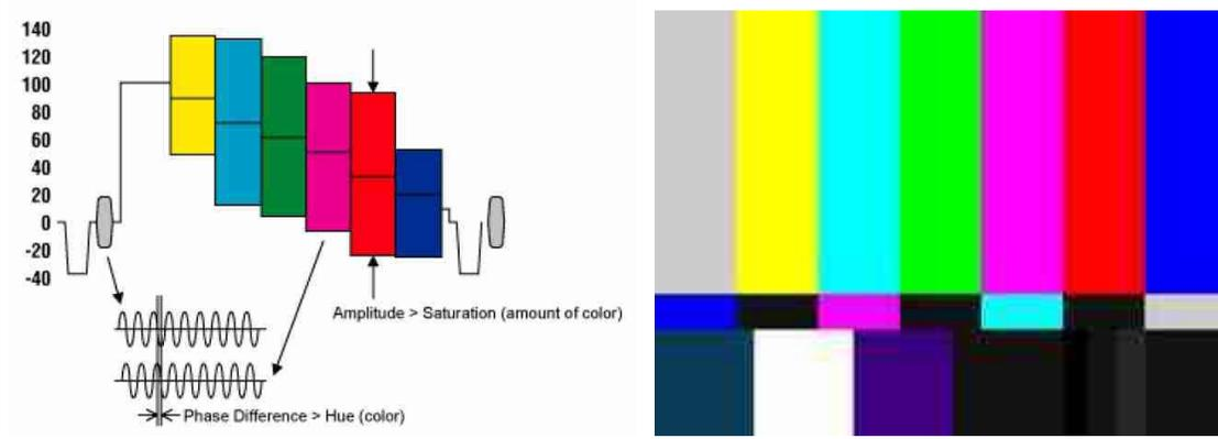
Fig. 3 Composite video signal with color bars & the resultant image on a video monitor.
