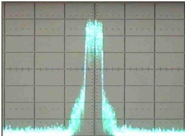
Fig. 13 Typical spectrum from an amateur DTV transmitter. 10dB/div &amp; 10MHz/div
