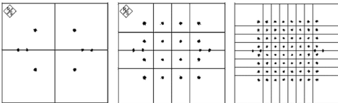
Fig. 14 DVB-T, I-Q Constellation Diagrams for QPSK, 16QAM AND 64QAM (left to right)
