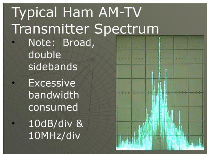
Fig. 10 Typical amateur AM-TV transmitter's spectrum
