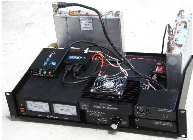
Fig. 27 A basic, 70 cm, 10 Watt, DVB-T, Television Repeater
