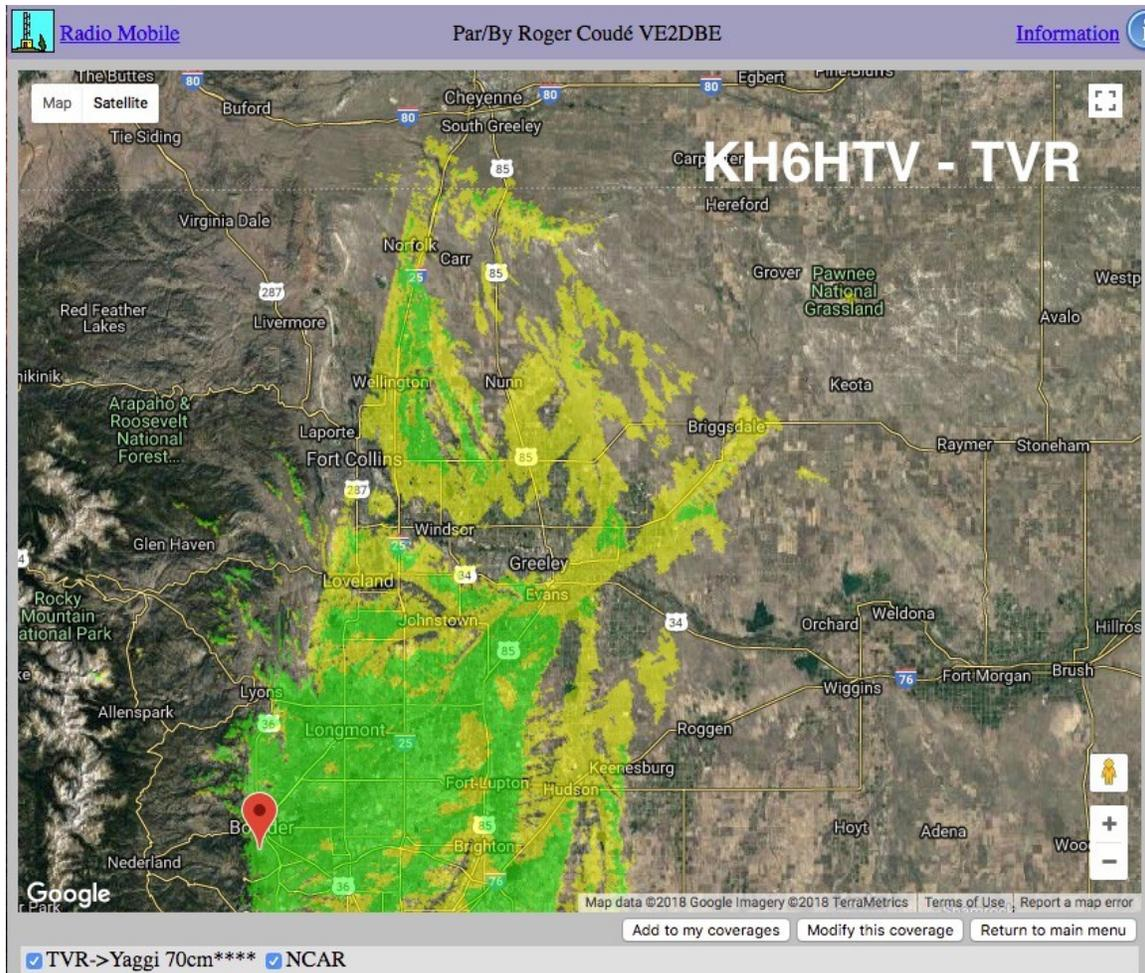
Fig. 26 Boulder, Colorado TV repeater coverage map generated by *Radio Mobile*.
