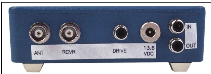
This rear-panel view of the 8-W Brickette shows compact but uncrowded I/O connectors clearly labeled.
