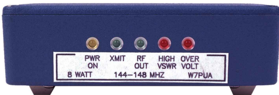
The five LEDs on the Brickette’s front panel signal the amplifier’s operating status. The power-output (RF OUT) and SWR (HIGH VSWR) LEDs vary in brightness depending on the forward and reflected power levels.
