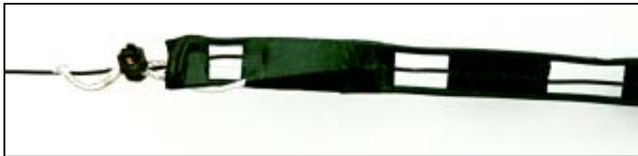
Figure 6 — There are several ways to secure the end of the ladder line to the #12 wire. I chose electrical split-bolt connectors with nylon cord for mechanical strain relief. Care should be taken to insure that the shorted end of the ladder line does not come in contact with the wire.
