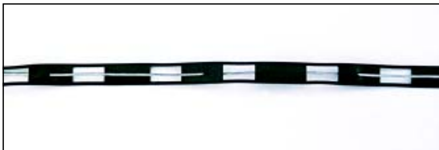
Figure 3—Final assembly method using interlaced #12 Copperweld wire through holes punched in the windowed ladder line.
