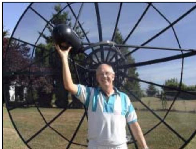
Fig 6—W7SZ with his dish antenna used on 10 GHz. The microwave equipment is mounted at the focus of the antenna. Equipment for 10 GHz is similar to that used by W7LHL except that the transmitter power amplifier uses a TWT (traveling-wave tube).
