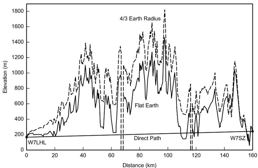
**Fig 3—Cross section of the terrain between W7LHL and W7SZ. It is far from a direct path. The tallest peak, shown at about 100 km from the W7LHL end, is the side of Mt St Helens. The upper trace shows the effect of the Earth's curvature, including a 4/3 correction for refraction. The "Flat-Earth" trace is about 400 meters lower in the center of the path. (Plot by KB1VC; users.rcn.com/acreilly/los\_form.html)**
