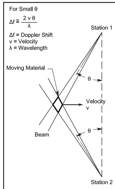
**Fig A—Geometry for observing the Doppler shift on a signal that has been scattered by a moving media. The antenna beams have been shifted off the direct path. Angles are in radians, which are about 0.01745 times the angle in degrees. The distance units for velocity and wavelength should be the same and the velocity should be in distance units per second. Then the Doppler frequency shift will be in hertz. This geometry is specific to a path at right angles to the moving media.**
