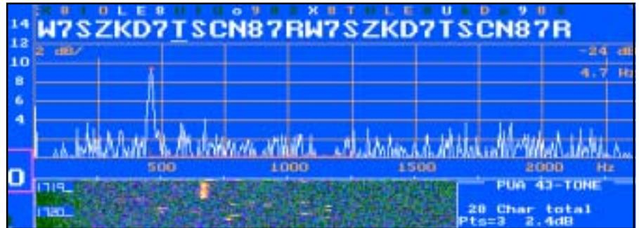
Fig 7—Partial screen shot of KD7TS's 10-GHz signal being received at W7SZ. The top lines of text show the most likely (large letters) and the second most likely characters being received in PUA43 mode. Below the letters is the latest spectrum of the multitone FSK signal. A portion of the waterfall display appears at the bottom.
