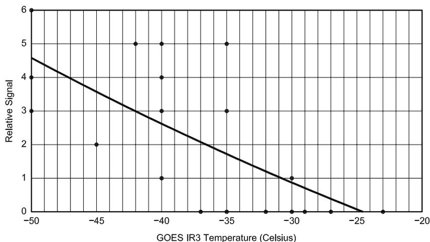
Fig 12—This plot shows the correlation between the GOES-10 IR3 temperature and the received 10-GHz signal strength over the W7LHL/W7SZ path. See the text for the meaning of the relative signal strength. Each of the 19 dots represents a different day’s measurement. The straight line in the plot is a linear curve fit to the data, showing the trend between temperature and signal strengths.
