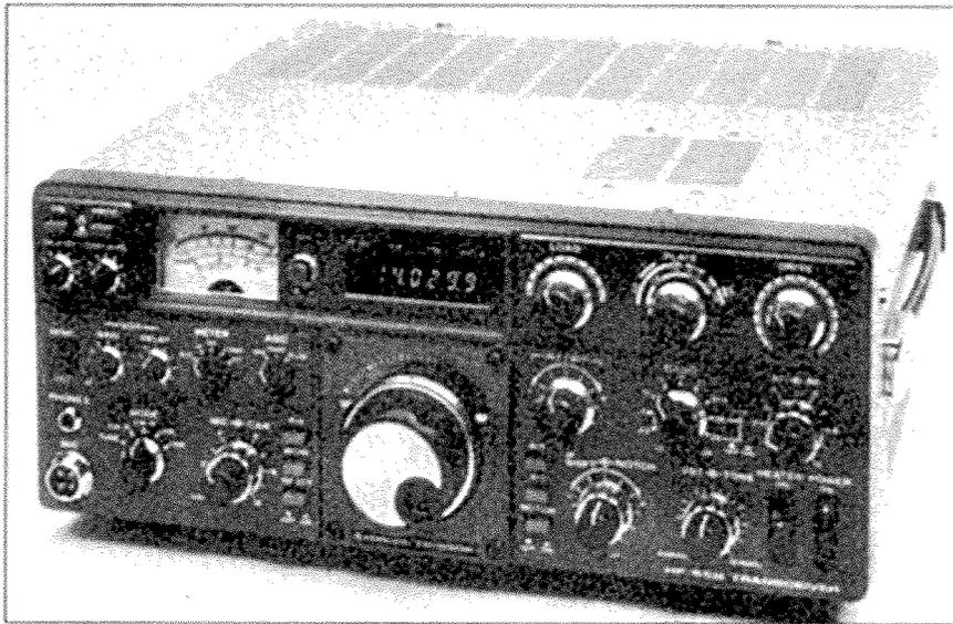
**The Kenwood TS-830S transceiver is mostly solid state. The final-amplifier tubes are commonly available 6146Bs. If you think you might want to work split-frequency (for DXing), look for a TS-830S that includes one of the two optional remote VFOs. This transceiver does not include a general-coverage receiver.**
