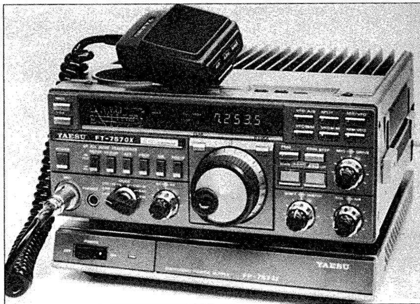
Yaesu's FT-757GX also packs a lot of radio in a small box. For CW fans, this radio features full break-in CW and a built-in keyer. Optional interfaces allowed computer frequency control. The '757GX in this photo rests on an optional, lightweight switching-mode power supply. Look for a 13.5-V dc, 20-A supply for home use.
