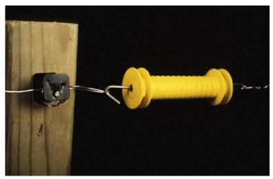
Gate hooks are a potential problem. They often become corroded where they contact the wire, resulting in an arc or
