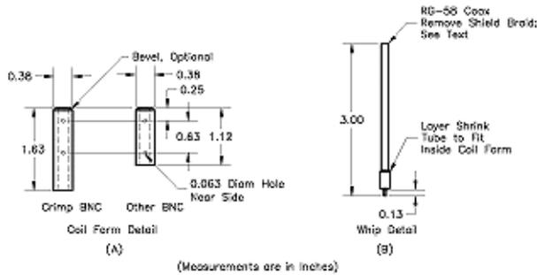
**Figure 1—Making a replacement H-T antenna is relatively simple. The details show the dimensions and cross-sections of the coil form (A), whip (B), and the initial and finished stages of antennas (C) made with three types of BNC connectors: standard, crimped and molded.**
