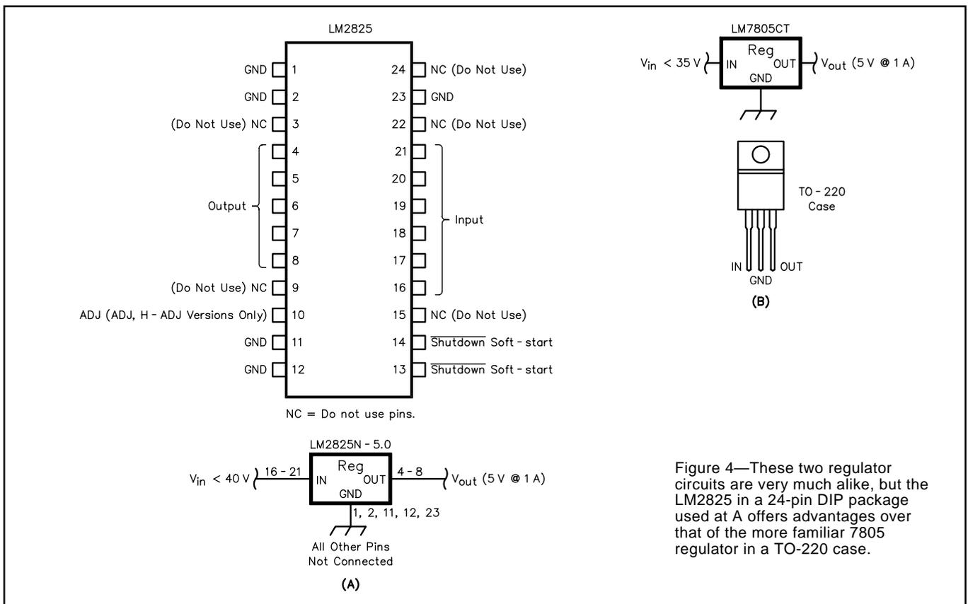
Figure 4—These two regulator circuits are very much alike, but the LM2825 in a 24-pin DIP package used at A offers advantages over that of the more familiar 7805 regulator in a TO-220 case.
