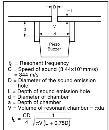
Figure 19—Here's the fundamental approach to constructing a resonator to improve the loudness and purity of the buzzer's tone. The resonant frequency ( $f_0$ ) should equal twice the frequency of the buzzer to increase sound pressure. Do not make dimension D too small, or the acoustic resistance will increase. The equation is a starting point; experimentation will optimize your results (see text). Dimensions are in millimeters unless otherwise noted.
