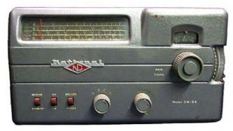
The 1950 SW-54 was one of the few models of ac -and dcpowered receivers made by National. [Photo courtesy of www.radiopics.com]
