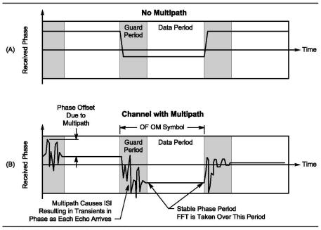
Fig 11—ISI Rejection using Guard Band
