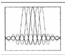
Fig 1—OFDM carrier interleaving.
