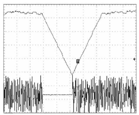
Fig 12—Synchronization with Normal REF Symbol
