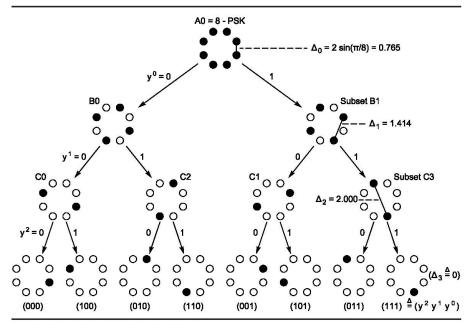
Fig 5—Signal Constellation Partitioning
