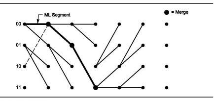
Fig 8—Viterbi Decoding
