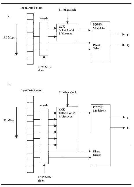
Fig 2—Encoding complementary code frequency sequence.
