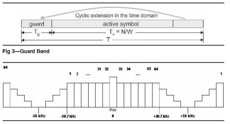
Fig 4—Format for 125 kHz Channel Spacing
