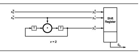
Fig 6—Convolutional Coding
