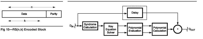
Fig 16—RS Error Correction Process
