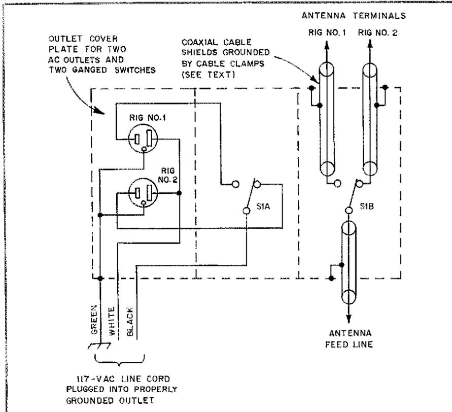
Fig 3—Power and antenna switching for two rigs.
