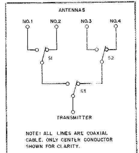
Fig 4—Three toggle wall switches used to select one of four antennas.
