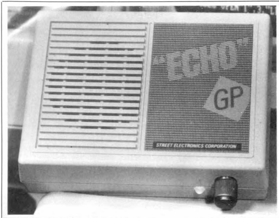
Fig 4—The Echo GP external speech synthesizer. This unit has a built-in text-to-speech converter and is driven by the computer through a serial communications port.
