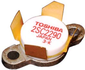
Figure 5—Detail of bending of the power transistor connections.
