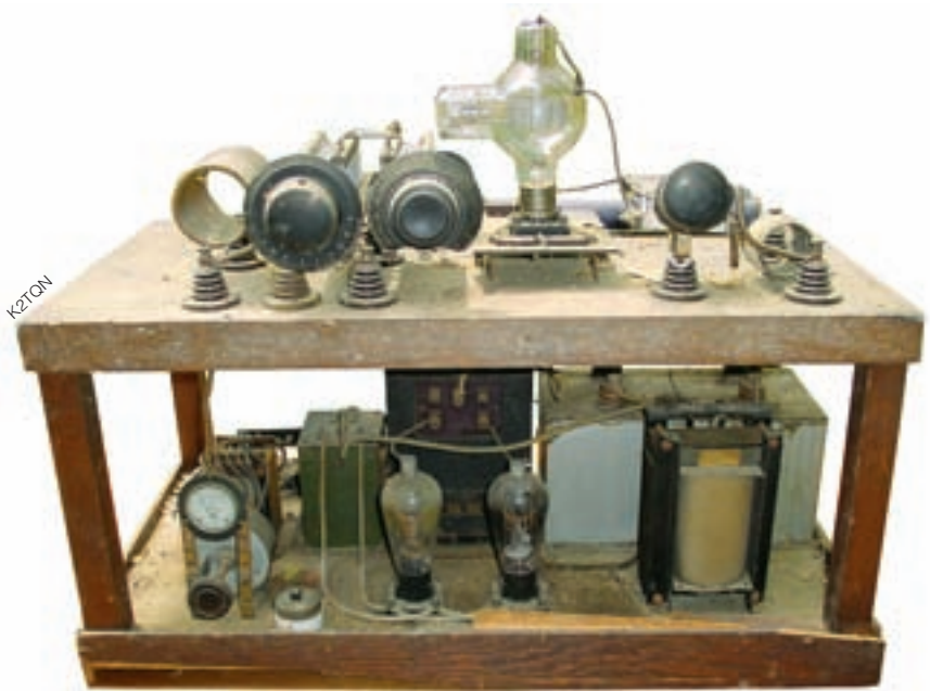
Transmitter as found with broken knobs, insulators, and 52 tube plate lead and broken trim moldings.
