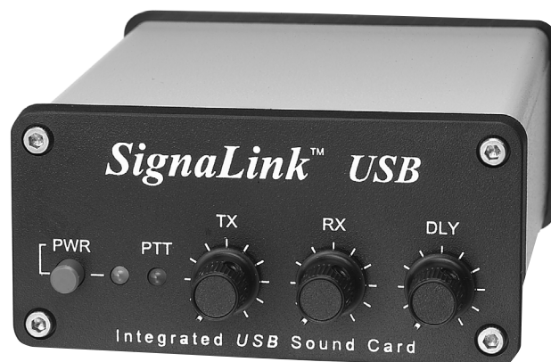
The Tigertronics Signalink is typical of the devices known as “sound card interfaces.” It allows your computer to switch your transceiver between receive and transmit. It also provides isolation for the audio lines.
