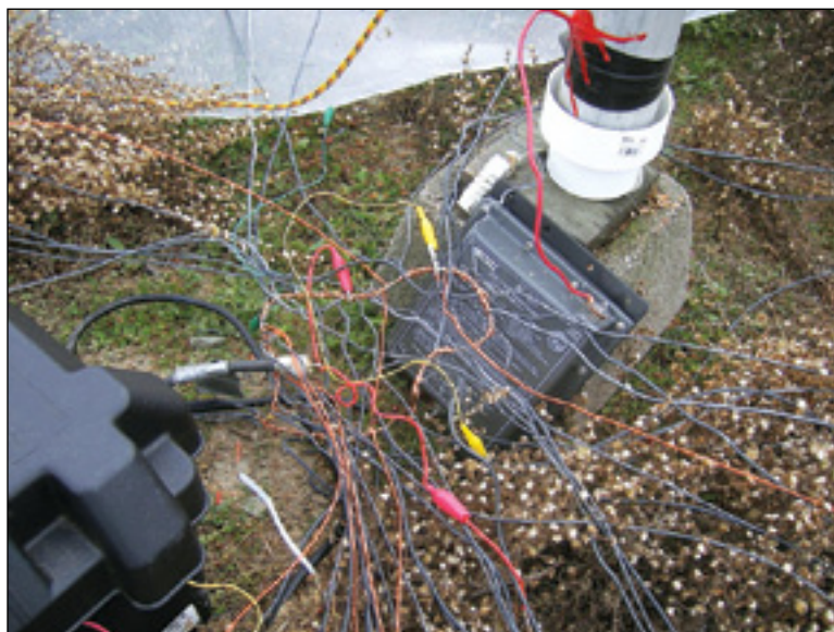
Like many portable operations, Jim’s, K6EI, antenna wiring lash-up wasn’t pretty but it worked. This is the base of his temporary 70 foot inverted L with 52 radials and an SGC-237 remote tuner. Jim worked 275 stations and 58 multipliers to lead the Pacific Division in the Single Operator, QRP category. [Courtesy Jim Peterson, K6EI]
