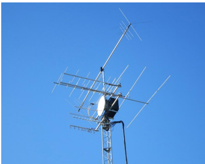
A better view of the N6NB antennas for 14 bands, 7 MHz through 10 GHz (photo courtesy Gregory Campbell, W6IT)
