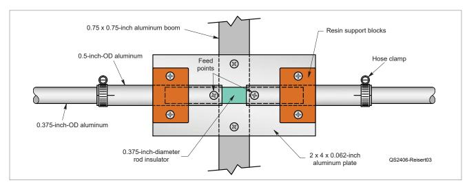
Figure 3 — Driven element construction details.
