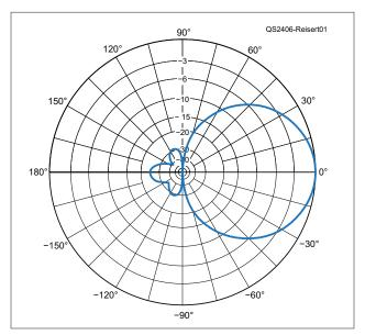
Figure 1 — The *NEC* calculated pattern for the 2-meter Yagi, redrawn for clarity. The front-to-rear ratio is very good.
