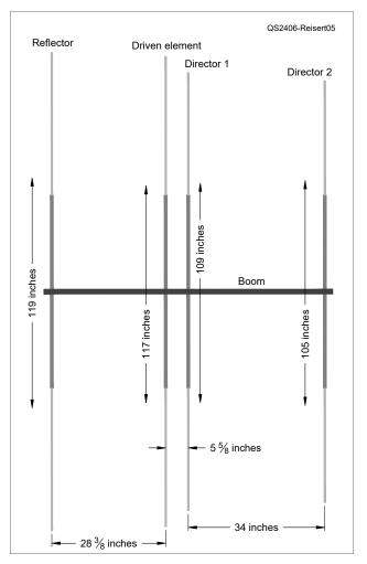
Figure 5 — Dimensions of the four-element, 0.29-wavelength 6-meter Yagi.
