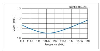
Figure 4 — Voltage standing wave ratio (VSWR) versus frequency, as calculated by  $\it NEC$  and redrawn for clarity.
