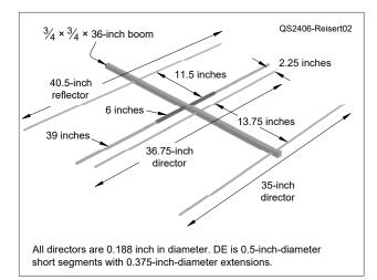
Figure 2 — Dimensions of the 2-meter Yagi.
