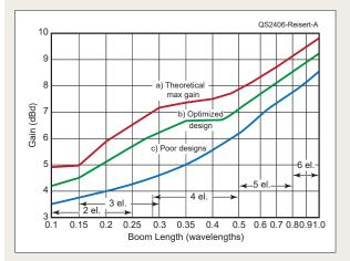
A graph of the actual gain attainable and the recommended number of elements versus the boom length for a Yagi. The upper curve is the maximum gain attainable if other parameters are sacrificed. The middle curve shows an optimized Yagi. The lower curve represents a poor performance design.
