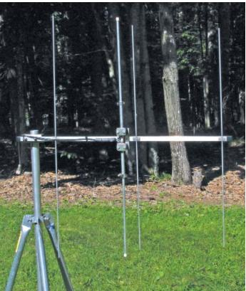
The 2-meter Yagi mounted in the vertical polarization. [Joe Reisert, W1JR, photo]  $% \left[ {{\left[ {{{\rm{N}}_{\rm{T}}} \right]}_{\rm{T}}} \right]_{\rm{T}}} \right]$
