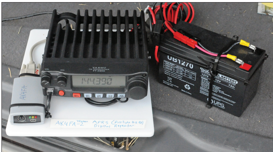
Figure 4 — The 75 W digipeater in the back of a vehicle during testing. The Microsat PLXdigi (small white box on the left) provided reliable digipeating for the event.
