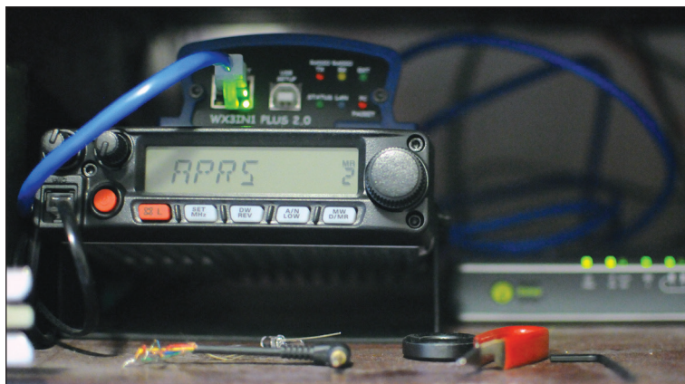
Figure 3 — The last leg of the APRS infrastructure that bridges radio to the Internet is the iGate. The iGate remained at my home, where it picked up packets from the event digipeaters and forwarded them to the APRS servers using my Internet connection. The Microsat WX3in1 Plus 2.0 iGate performed flawlessly during the event.
