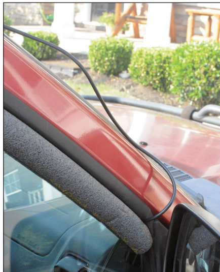
Figure 6 — Routing antenna and GPS cables in borrowed vehicles can be challenging. To avoid shorting the coax by closing the door on the cable, we used pipe insulation over the window glass to create a moisture and air barrier without damaging the cables.
