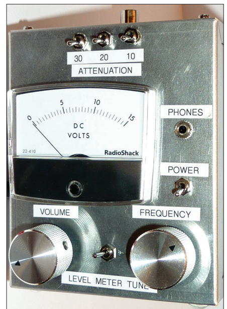
Figure 5 — Noise receiver front view.
