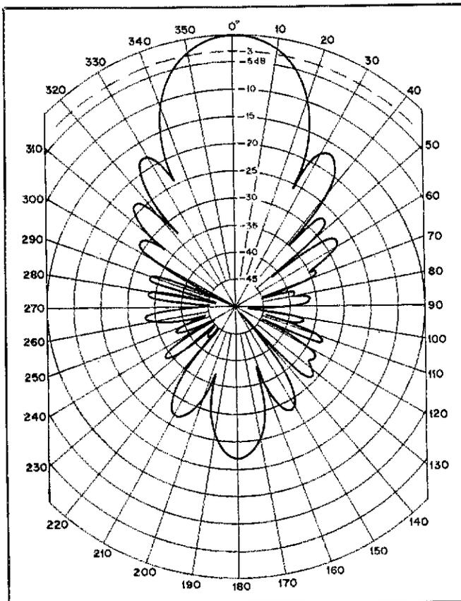
← Fig 2—Measured E-plane pattern for the K1FO 22-element Yagi. Note: This antenna pattern is drawn on a linear dB grid, identical to the grids in Fig 1, rather than the standard ARRL log-periodic grid.
