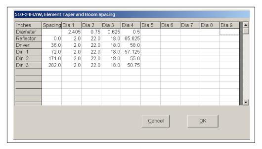
Fig 12—Elements window for 510-24H Yagi.
