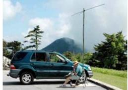
KB5YZG on his first VHF outing using an ICOM-706, with an 11 element yagi on top of a stack of fiberglass tent poles. Car battery provided talk power, elbow provided rotor power.
