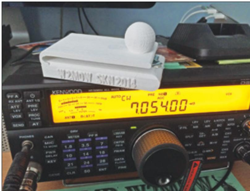
Matt Williams, W2MDW, put a 21st-century twist on SKN, using a straight key he made with his 3D printer. Matt modeled the key a few days before the event, which is why "2014" is printed on the key. You can learn how to make your own straight key with a 3D printer thanks to an article Matt has penned for an upcoming issue of *QST*. [Matt Williams, W2MDW, photo]
