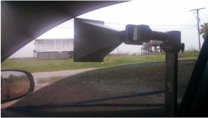
Al, W5LUA operating on the Gulf Coast in the rain. Note the drop of water hanging off the bottom right side of Al's secondary antenna - a horn. This was during two successful 424 km contacts! (Photo credit – Al Ward, W5LUA)
