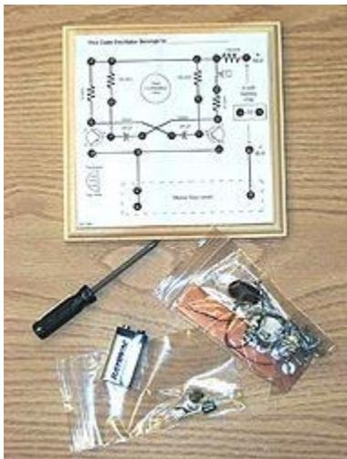
The breadboard is pre-drilled, and the edges are nicely routed. For a complete kit, the club even includes a Phillips screwdriver--so students can get going right away, and teachers can avoid an additional out-of-pocket expense.
