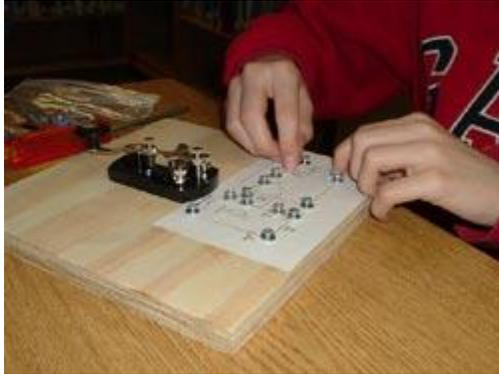
**With the wood screws and washers mounted, the process of connecting the components begins.**
