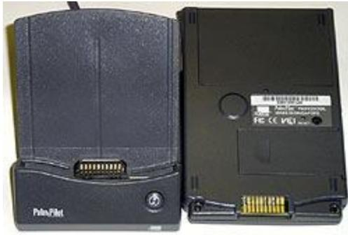
In my case I wired in and secured a 10-pin plug so that I could continue to interface the Palm to the docking cradle and also connect the Palm to the SureLink transceiver and supporting circuits.
