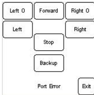
Basically the Palm software displays directional keys on the screen and opens the serial port of the Palm to the SureLink transceiver. When the user touches one of the control buttons, a command represented by a letter is placed in a transmission cue awaiting a signal from the BOE/BOT that it is ready to receive the command. Once the go-ahead is received, the Palm sends the command to the SureLink for transmission.
