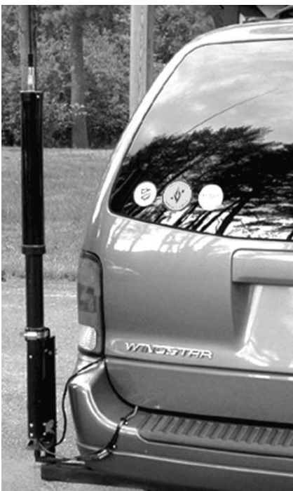
The High Sierra HS-1800 is a so-called “screwdriver” style HF mobile antenna that provides continuous coverage for all HF bands.
