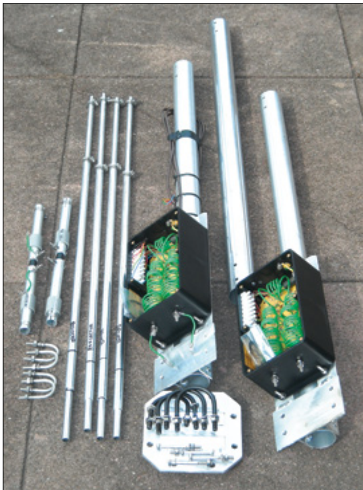
Figure 5 — The pieces of the antenna as delivered. All pieces are 3 feet or shorter, making the Q-52 easy to transport for portable operation. Total weight of the antenna is 16 pounds.
