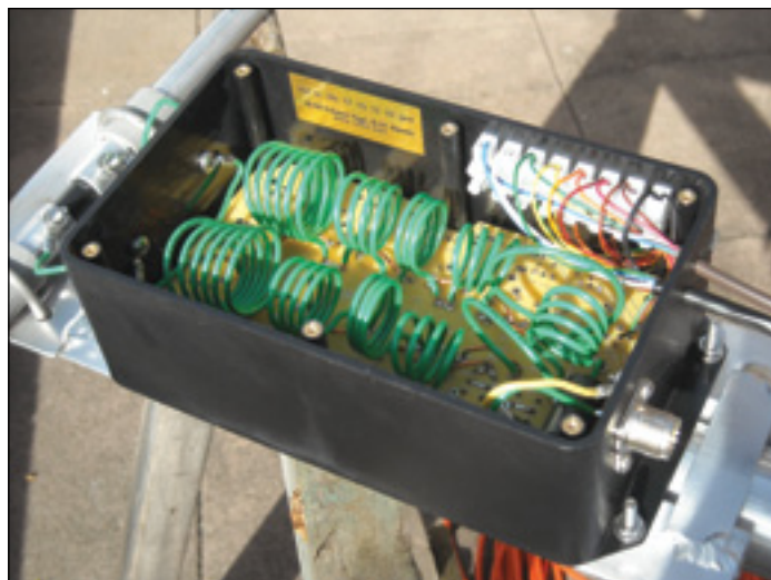
Figure 4 — The driven element's relay and inductor assembly with the control cables to the shack and to the reflector element attached to the terminal strip.
