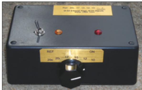
Figure 3 — The Q-52 control box has a single rotary switch for band selection and a toggle switch to open the reflector element for bidirectional mode.
