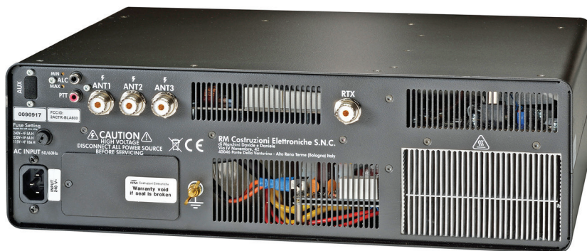
Rear panel of the BLA600, showing available connections. See text for details.
