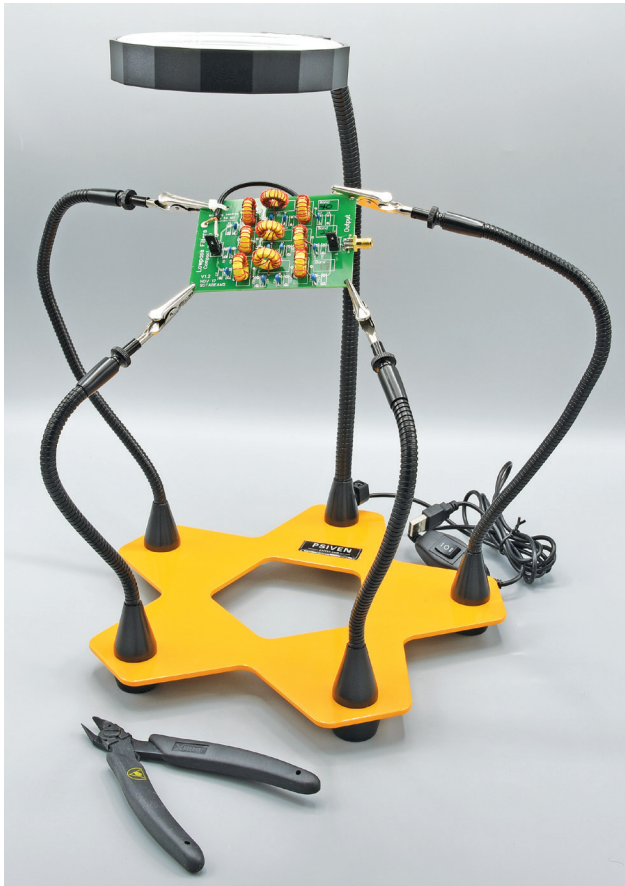
Figure 12 — The PSIVEN Helping Hands Third Hand Soldering Tool and Vise has four alligator clips and a magnifying lens with an LED light source, giving a lot of meaning to the word “flexibility.”
