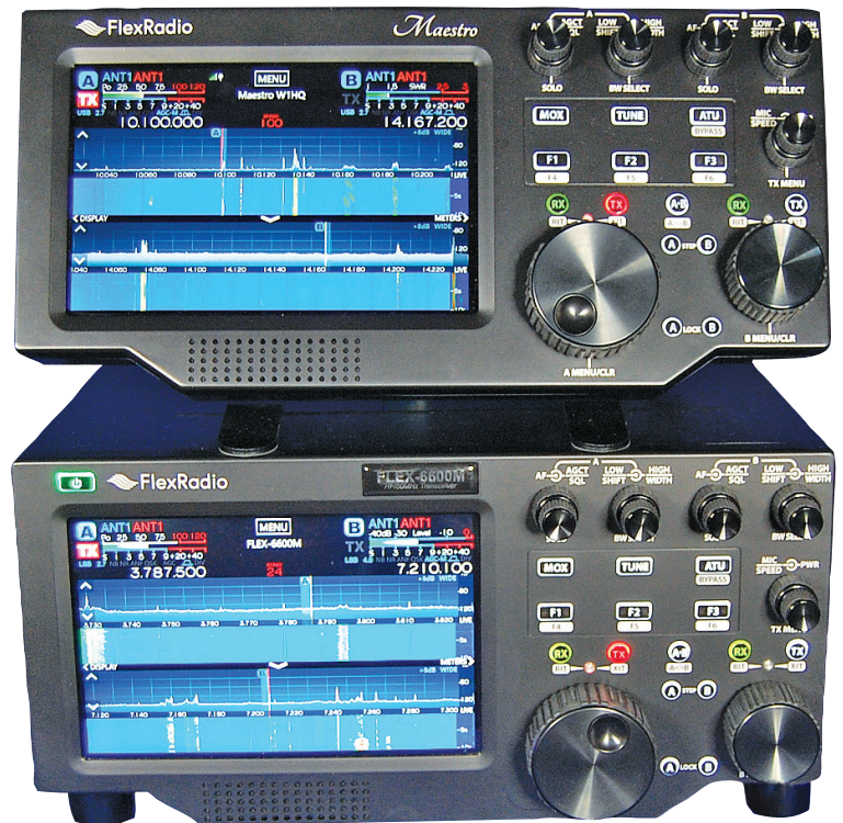
Figure 1 — MultiFlex operation with a Maestro (top) and FLEX-6600M transceiver connected to a single antenna. The Maestro receives 30 and 20 meters, while the FLEX-6600M receives 80 and 40 meters.
