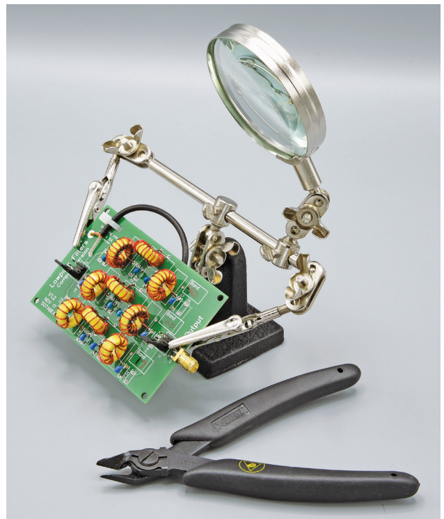
Figure 9 — The classic and inexpensive Helping Hand design is available with and without a magnifier.
