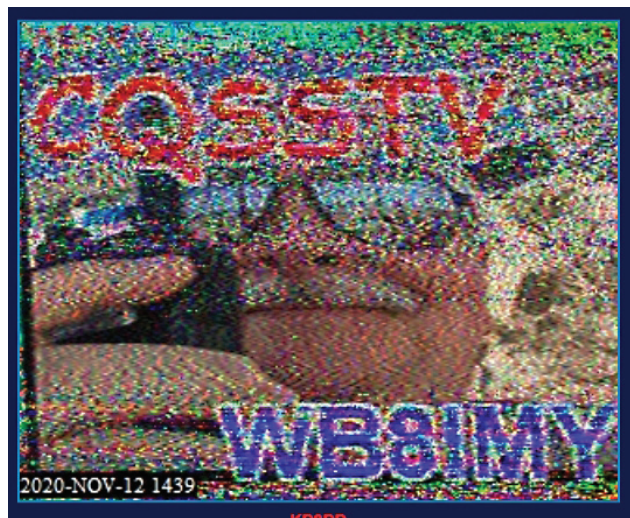
Figure 4 — You can attach an external computer and operate slow-scan TV (SSTV) with the IC-705. KD9DD was 1,000 miles away in Illinois, but he was still able to view my noisy 5 W CQ image.
