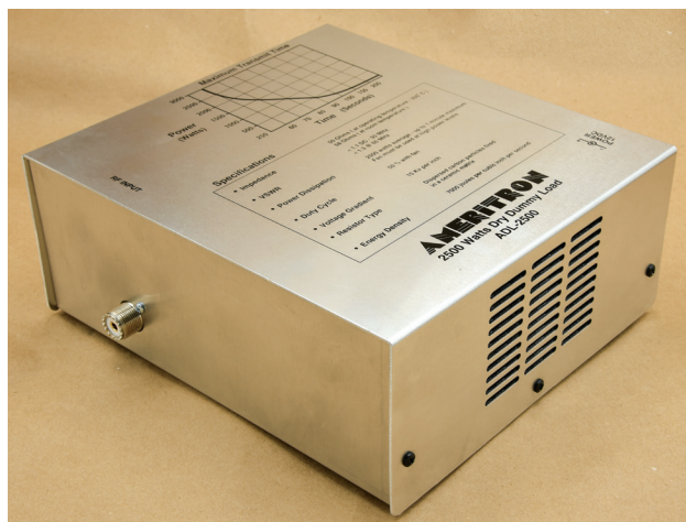
Figure 7 — The Ameritron ADL-2500 power-handling chart and specifications are printed on the top of the case.
