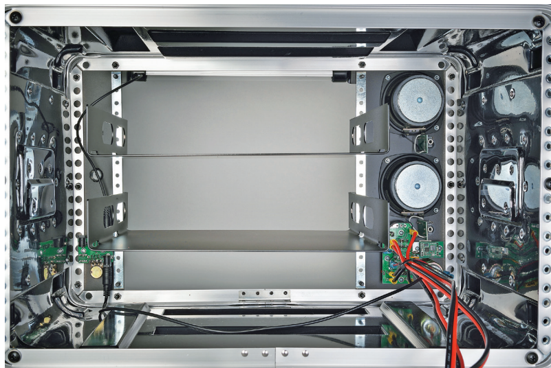
Figure 6 — A look into the rack case from the rear. The speakers and power wiring are visible on the right side.
