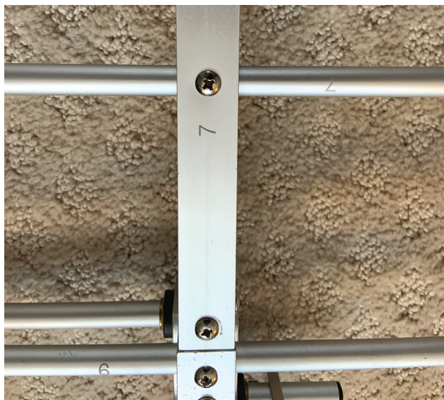
Figure 3 — Each element is inscribed with a number that corresponds to a matching number on the boom.
