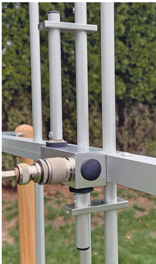
Figure 2 — The TC-YG08UV driven elements use individual gamma-matching sections for each band. A single feed line runs to the transceiver.
