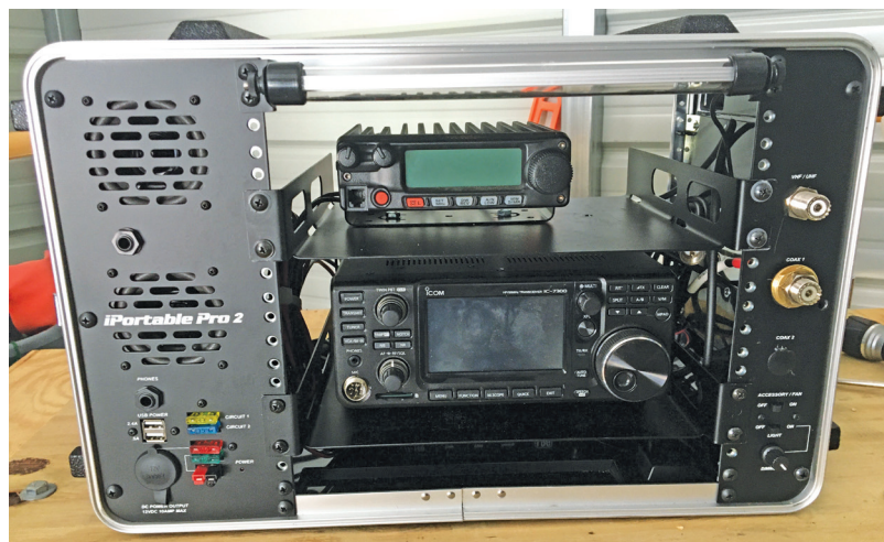
Figure 8 — The author's final configuration with an IC-7300 and an FT-2980R VHF FM radio in place.
