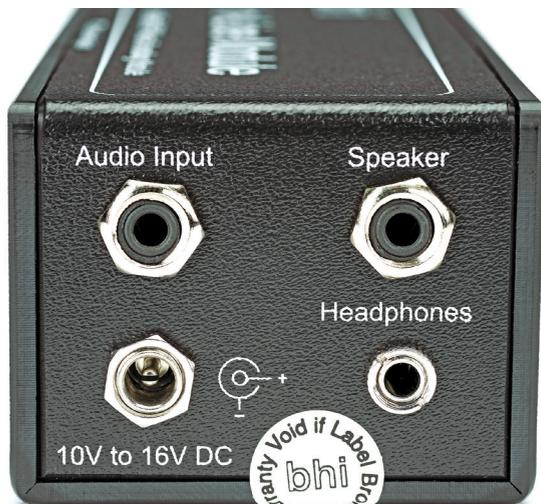
**Figure 6** — Input, output, and power — these are the only needed connections. You can choose an output to a speaker or headphones.
