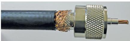
**Figure 12** — Inserting a PL-259 at the end of the stripped coax, with the coax shield above the bottom part of the connector.
