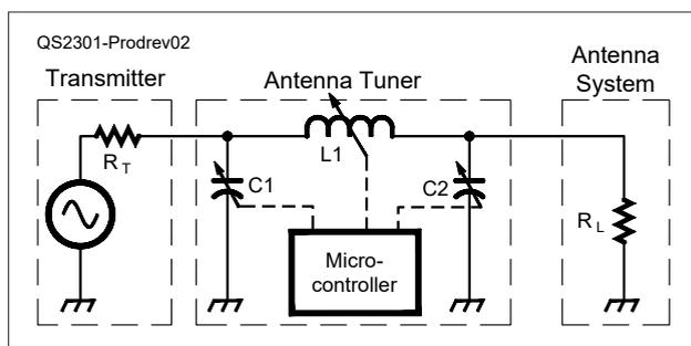
Figure 3 — Tuner Genius circuit. [Courtesy of FlexRadio]
