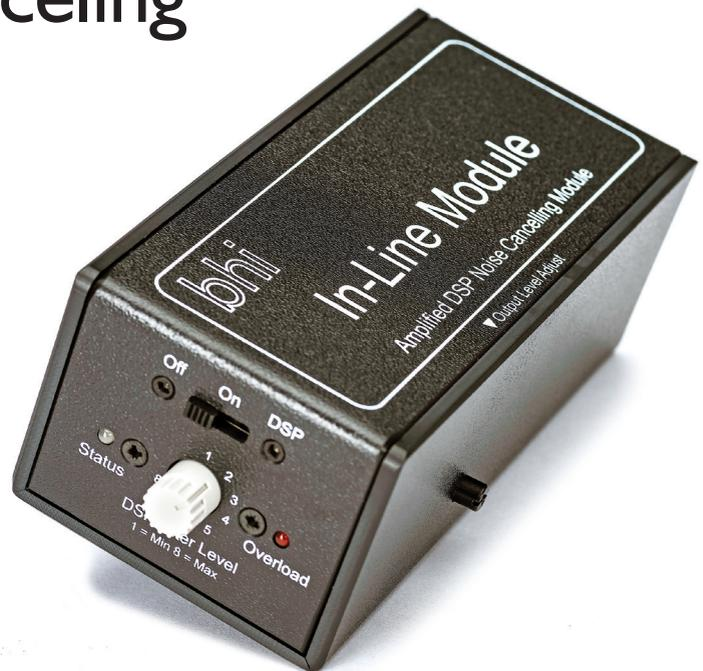
in voiding the warranty. The top left jack accepts a standard 3.5-millimeter monaural plug. Enclosed with the unit is a cable that has this mating plug on both ends — one end for the In-Line Module and the other end for the external speaker output of your receiver. Just below, on the left, is a 2.1-millimeter barrel connector for
