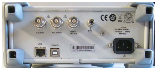
Figure 7 — The SIGLENT SDG 1032X rear panel. PC, LAN, and other input/output connections are made through this set of connectors.
