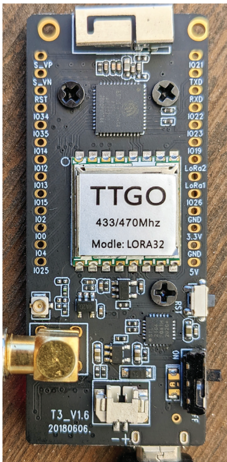
TTGO LoRa ESP32 board.
