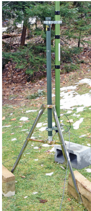
Figure 6 — The optional tripod mount uses the aluminum mounting pole that works with the hitch mount. I could not drive in the supplied 4-foot ground rods, so I secured the tripod with cement blocks. The antenna is lightweight, and it doesn't take much to keep it upright on a calm day.
