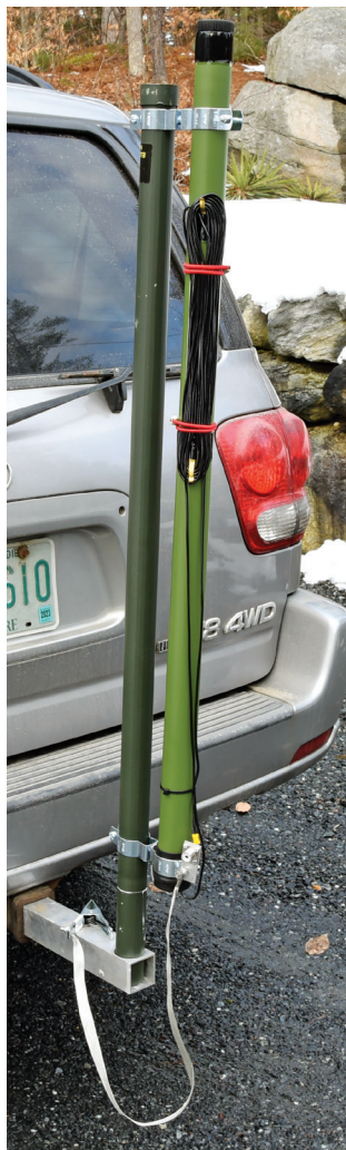
Figure 5 — The Eagle One antenna collapses to a 4-foot-long package for transport. It takes just a few minutes to install on the optional trailer hitch mount.
