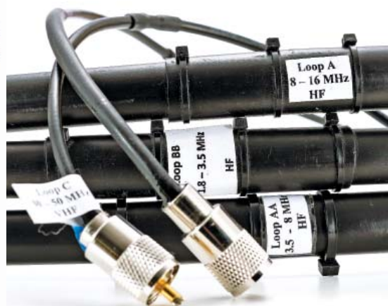
Figure 3 — Four of the five National RF loops, showing loops BB, AA, A, and part of C.
