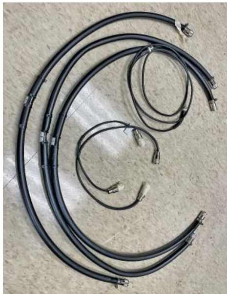
▶ Figure 5 — The National RF 3-foot interfacing cable with BNC connectors, a coax jumper, and three HF loops.
