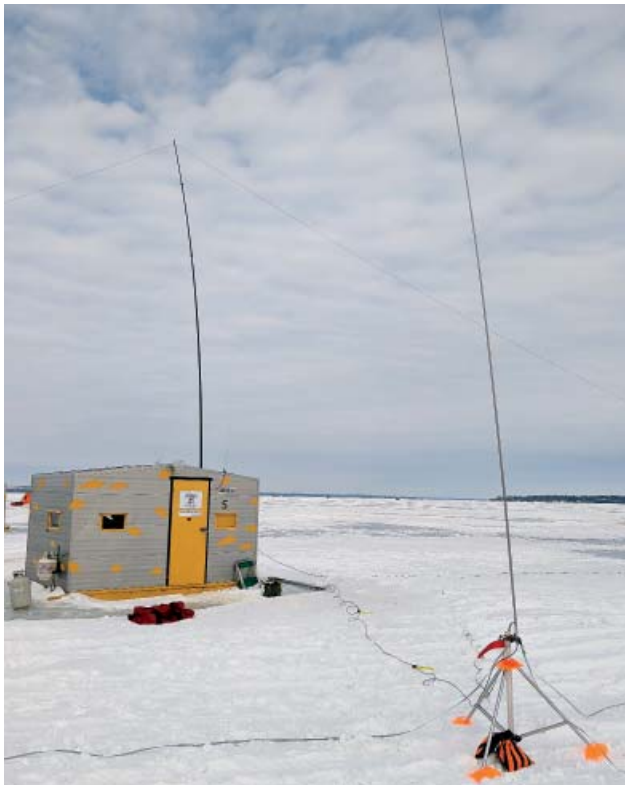
Figure 10 — The Chameleon Antenna MPAS 2.0 attached to an ice hut installation.
