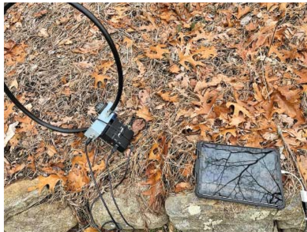
Figure 7 — The SDRplay SDR receiver attached to the National RF noise gun handle.
