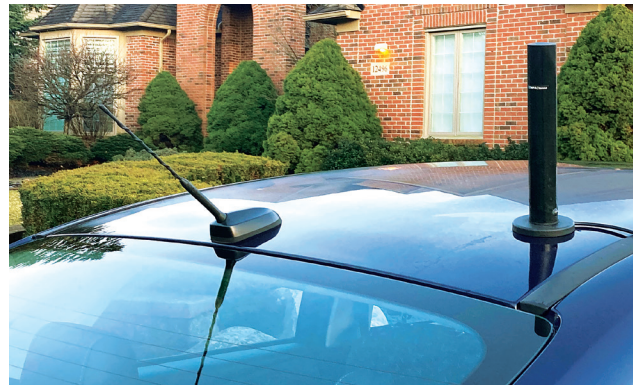
Figure 9 — The COMPACTenna 2M/440+ vehicle installation with the Larsen NMO magnetic mount.
