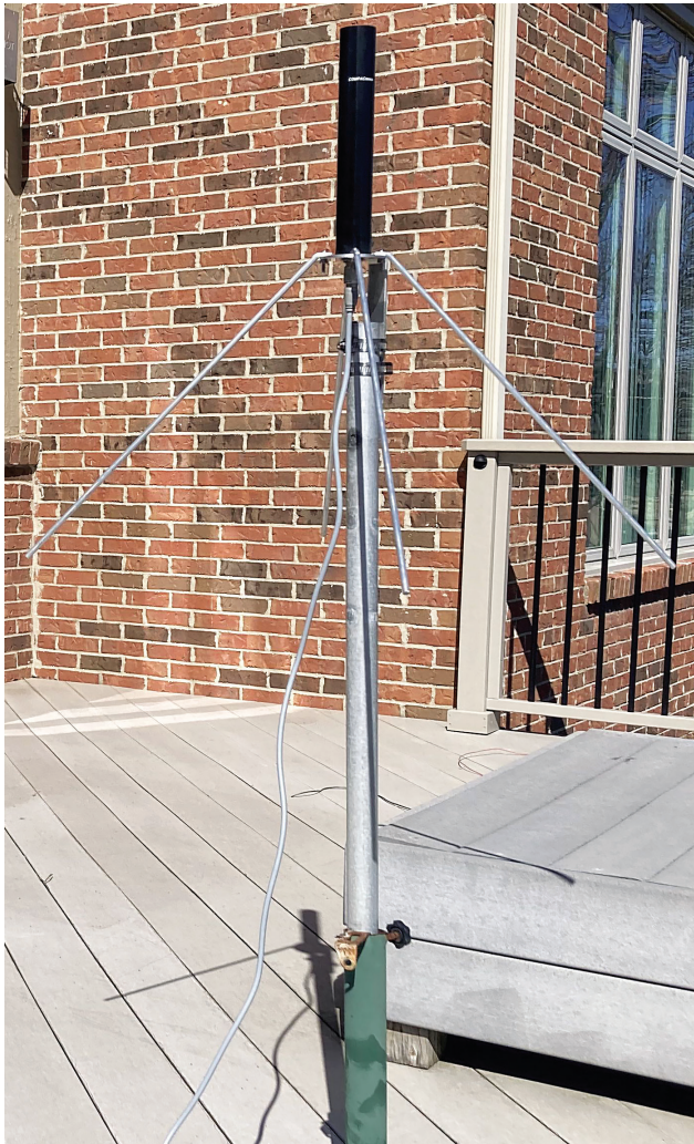
Figure 8 — The COMPACTenna 2M/440+ balcony station installation with CompacCounterpoise ground plane.
