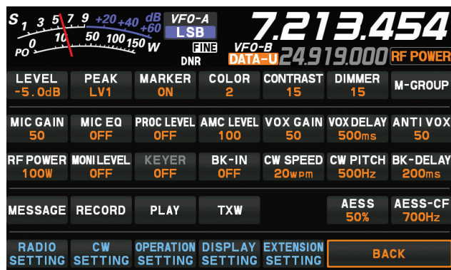
Figure 3 — Pressing the FUNC knob brings up a screen to access many of the radio's settings. Touch one of the onscreen labels, and rotating the FUNC knob adjusts that function even after the screen returns to normal operation. In this case, RF POWER is selected. The blue SETTING labels at the bottom bring up additional menus for parameters that are adjusted infrequently.
