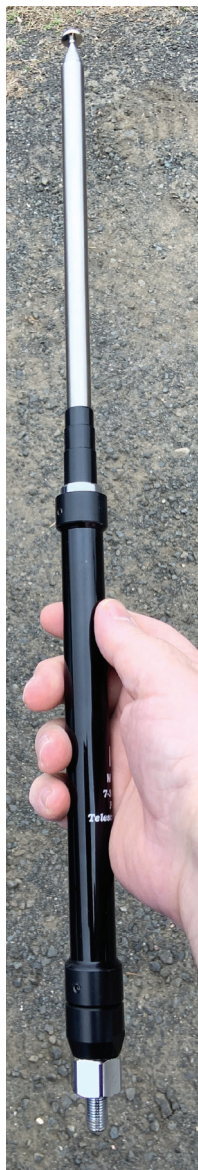
The MFJ-1898 is just 20 inches in length when the whip is fully retracted.
