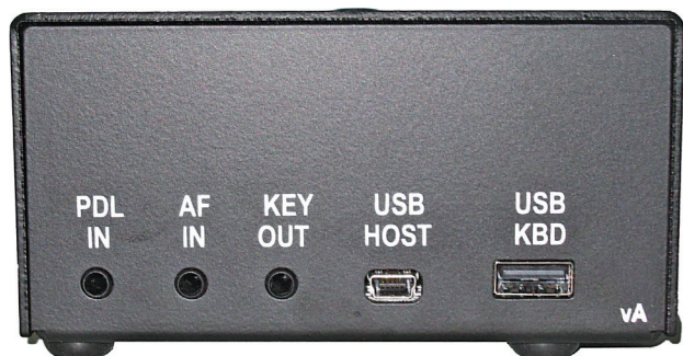
Figure 3 — Back panel connections. The three leftmost jacks accept 1/8-inch stereo plugs. A cable matching the USB host connector to a USB jack is supplied with the unit. A standard USB keyboard plugs into the right-hand socket.
