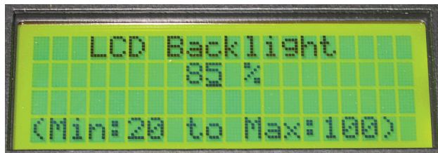
Figure 4 — Selecting the backlight control screen allows adjusting this value with the up/down arrow keys or the front panel rotary control.
