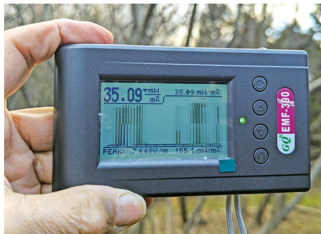
Figure 8 — The GQ EMF-390 measuring RF on 40 meters, and the “V V V” in CW is shown.
