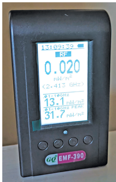
Figure 6 — The GQ EMF-390 showing Wi-Fi channel 1.
