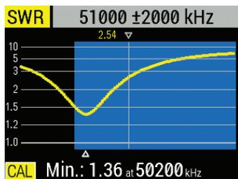
**Figure 8** — The Cushcraft ASQ-6 tuned SWR curve.
