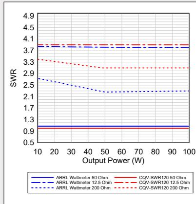
**Figure A** — The CQV-SWR120 power meter compared to the ARRL Lab wattmeter at 3.800 MHz.
