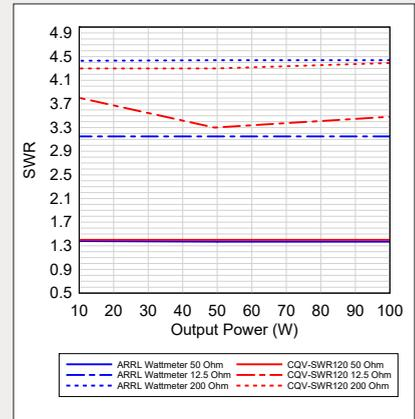
**Figure C** — The CQV-SWR120 power meter compared to the ARRL Lab wattmeter at 28.500 MHz.
