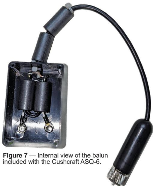
**Figure 7** — Internal view of the balun included with the Cushcraft ASQ-6.
