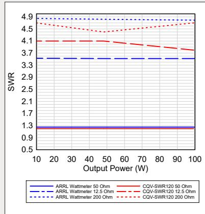
**Figure B** — The CQV-SWR120 power meter compared to the ARRL Lab wattmeter at 14.200 MHz.
